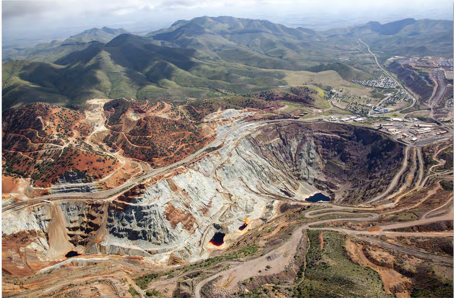
Figure 11-10: Only a fraction of ore mined is copper. A concentration mill is located close to the mine to increase the value per weight by removing non-copper rock from the ore.
